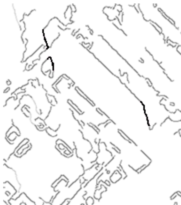
Figure 8. Detection of shadow edges collinear to metadata shadow angle.
