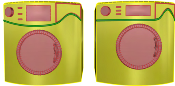
Figure 9: Semantic-mode: Altering the shape between two areas. Left: Old shape with a curvy coupler between the areas. Right: New shape with a less curvy coupler.
