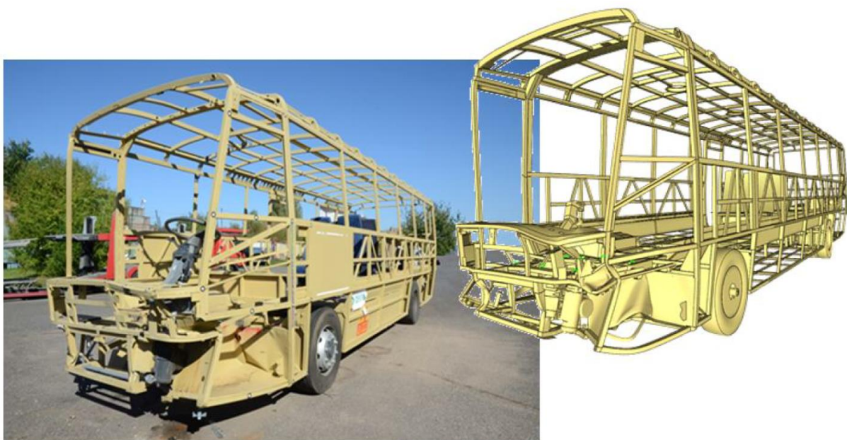
Fig. 1. Comparing computer simulation results with results of full scale test
