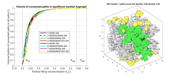
Fig. 1. Partical filling volume fraction of different materials and crystal sizes (left). An example of simulation model creation (right)
