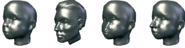
Figure 3.13: Undesired effects of naïve morphing. From left to right: Two input meshes, result of naïve morphing, morphing technique proposed by Alexa [1]. Source: [1]
