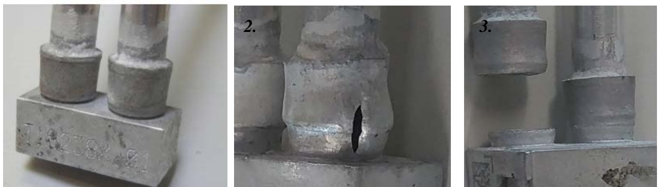
Figure 13-15: 1. Sample before test, 2. Test failure, 3. Test failure
