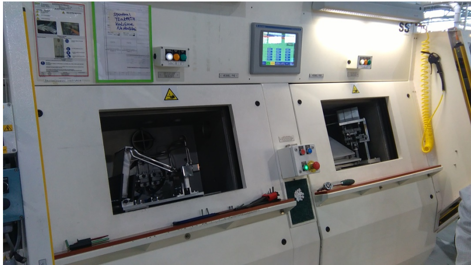
Figure 14-8: Leak tightness test in helium chamber
