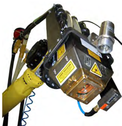
Obr. 4.1: HPDD laser Coherent Highlight ISL-4000L na robotu Fanuc M-710iC
