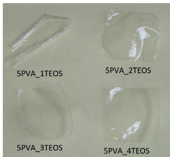
Figure 56. PVA/SiO 2 membranes after water uptake test.
