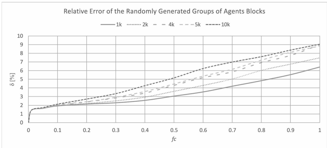
Figure 9. The average relative error \delta of the online computation for 100k generated agents in groups in dependence on facility cost fc
