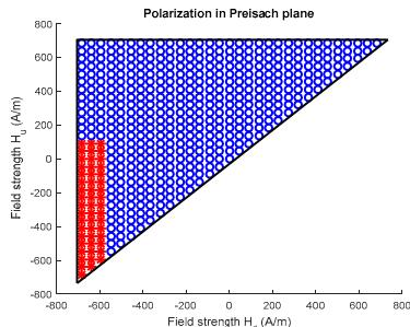
Figure 16. Preisach model for initial saturation.
