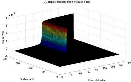
Figure 11. Magnetic flux in the Preisach triangle.
