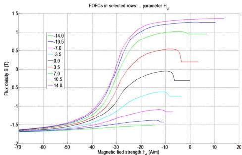
Figure 12. Magnetic flux density in the selected rows.
