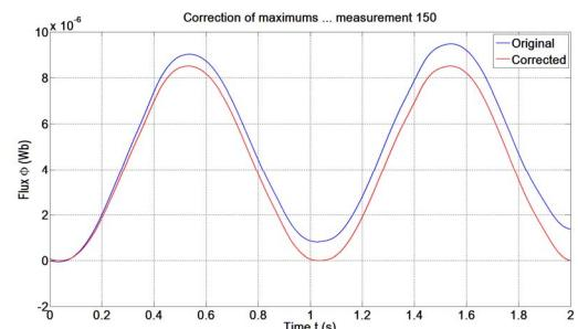
Figure 7. Elimination of the drift for low excitation.
