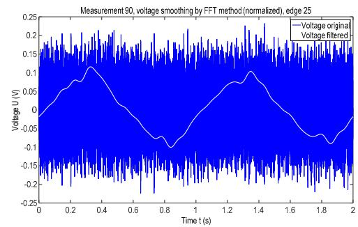
Figure 6. Filtering of the secondary voltage by FFT filter<sup>1</sup>.
