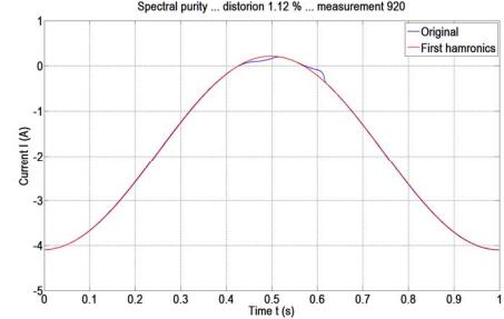
Figure 2. Current waveform deviation from pure harmonics.
