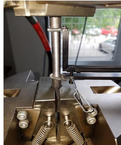
Fig. 1. Fastening of specimen with hydraulic wedge grips.
