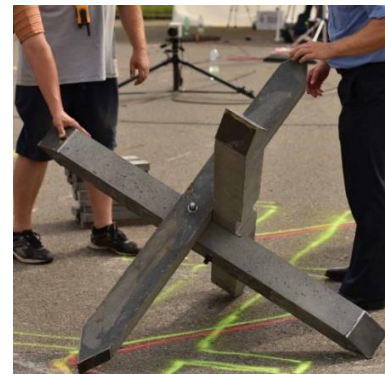
Fig. 1. The barrier for the first crash test.
