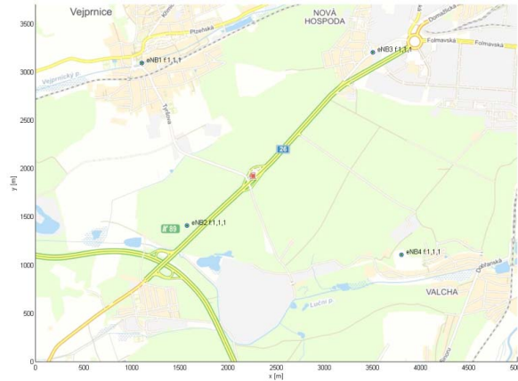
Fig. 7 Four eNodeBs were placed in the map in order to cover the whole area with sufficient signal
