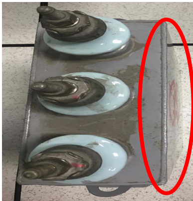
Figure 2. Expansion of power capacitor shell
