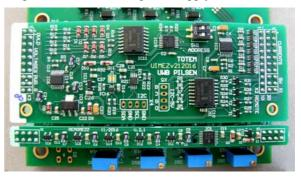
Figure 8. The remote access mezzanines. The U/I monitoring mezzanine (top) and the Remote Control mezzanine (bottom).
