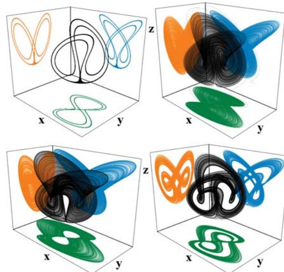
Figure 1. Three-dimensional perspective view on the numerically integrated typical strange attractor generated by Rucklidge system:  $a=2, b=4$  (upper left picture),  $a=2, b=6$  (upper right picture),  $a=1.3, b=6$  (lower left image) and  $a=1.3, b=4$  (lower right plot).
