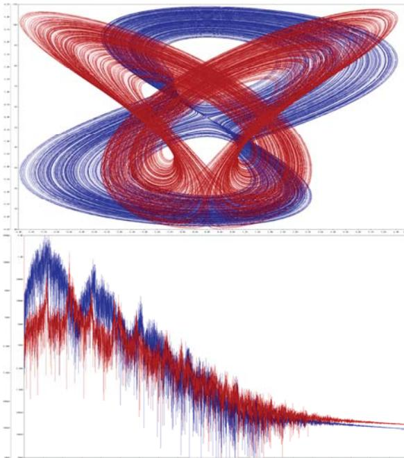
Figure 6. Orcad Pspice based simulation results:  $v_X$  vs  $v_Y$  (blue) and  $v_X$  vs  $v_Z$  (red) plane projection of the typical chaotic attractor (upper plots), generated chaotic signal  $v_X$  (blue) and  $v_Y$  (red) visualized in the frequency domain (lower plots).
