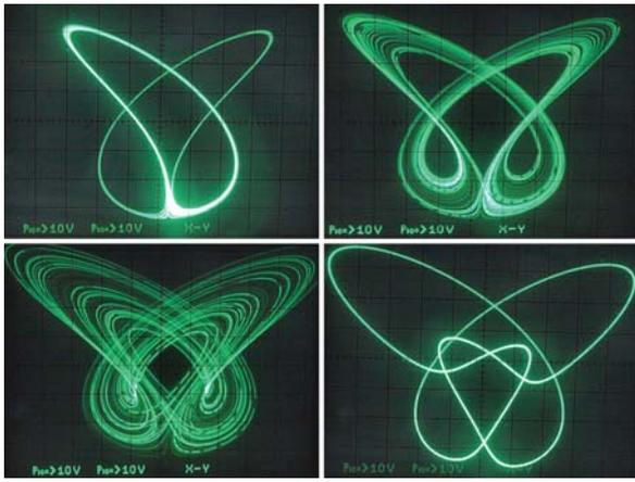
Figure 8. Measured state attractors plotted in  $v_X$  vs  $v_Z$  projection.
