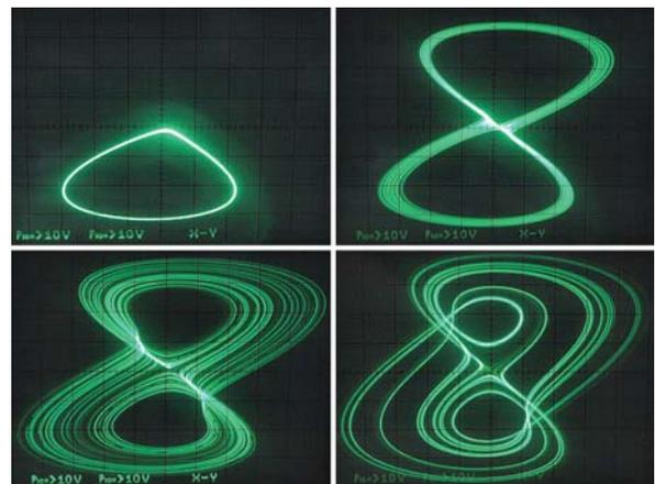
Figure 7. Measured state attractors plotted in  $v_X$  vs  $v_Y$  projection.
