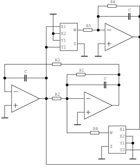
Figure 5. Circuitry implementation of Rucklidge dynamical system strictly following a concept of the analog computers.
