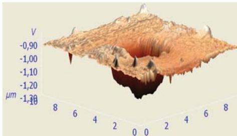
Figure 1. 3D potential distribution on the sample
