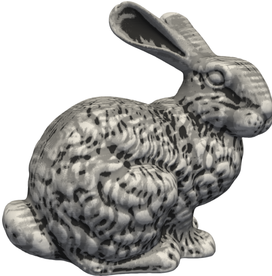
Figure 13: An isosurface of a CT scan of the Stanford Bunny colored using a grayscale mapping of hypersurface curvature classes.
