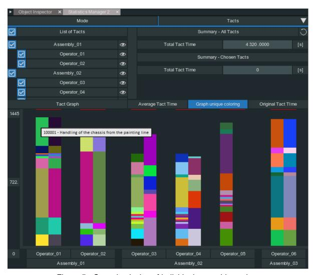
Figure 5 - Capacity design of individual assembly workers
