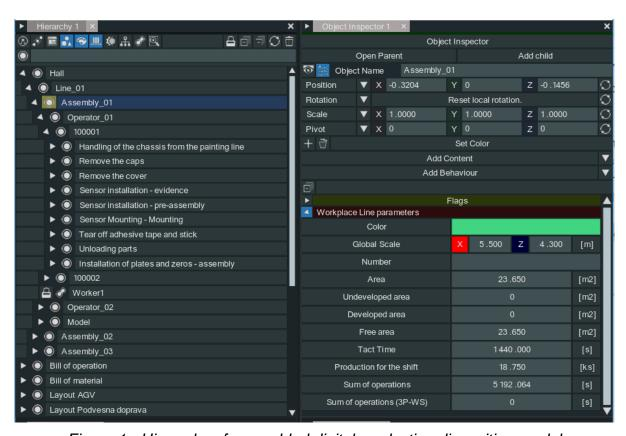
Figure 1 - Hierarchy of assembled digital production disposition model
