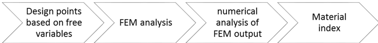
Fig. 1 Creating material index using FEM
