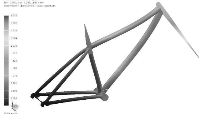
Fig. 6 Deformation and stress of HSS frame
