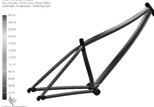
Fig. 6 Deformation and stress of HSS frame
