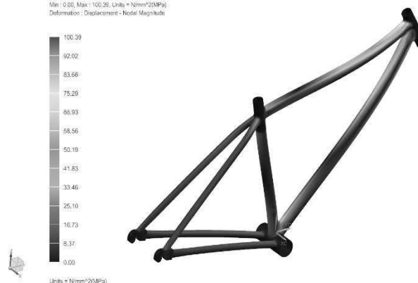
Fig. 5 Deformation and stress of aluminum frame
