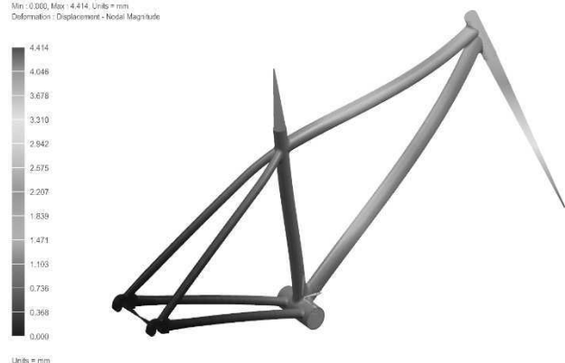
Fig. 5 Deformation and stress of aluminum frame
