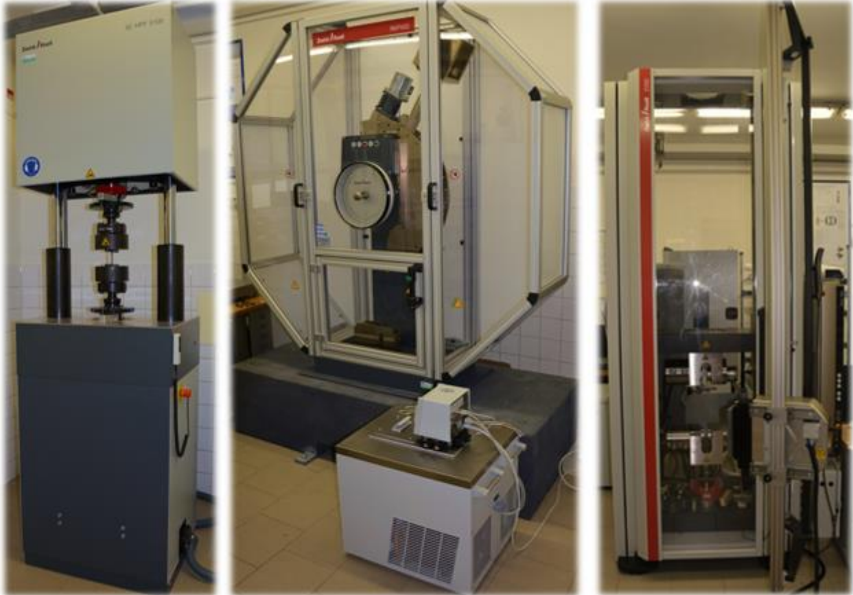
Fig. 1. Resonant pulsator (Zwick Roell HFP 50) – left, Hammer for impact test (Zwick Roell) – center, Universal tensile testing machine (Zwick Roell Z250 - right)
