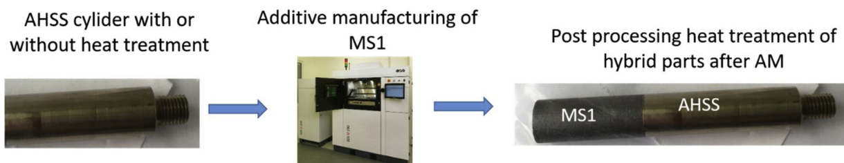
Fig. 2. Processing route with heat treatment combinations for used hybrid parts.
