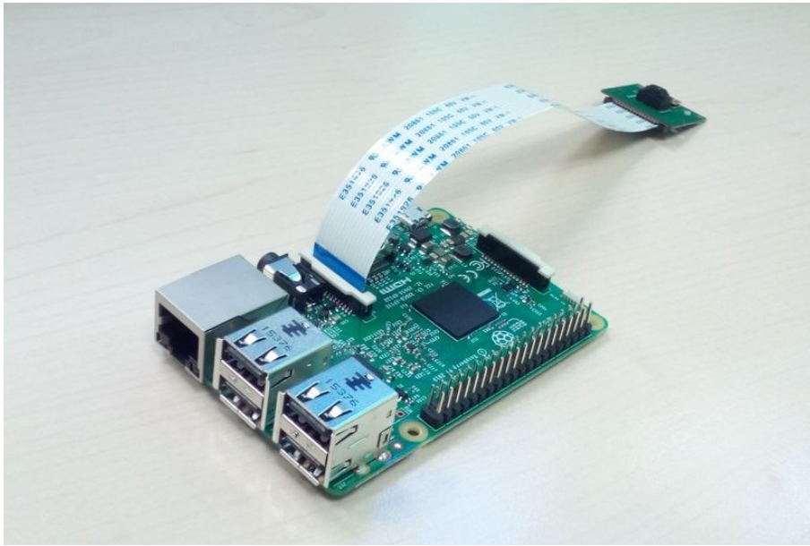
Figure 5.3: Camera module connected to a Raspberry Pi
