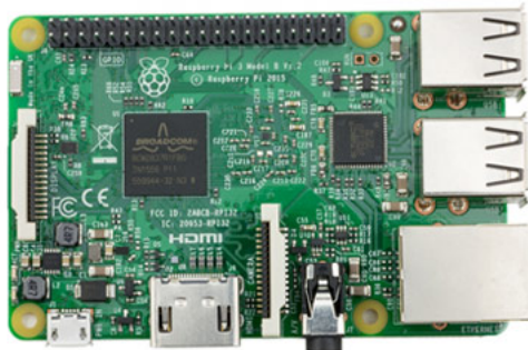
Figure 2.2: Raspberry Pi3 Model B+
