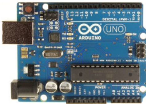
Figure 2.1: Arduino UNO board
