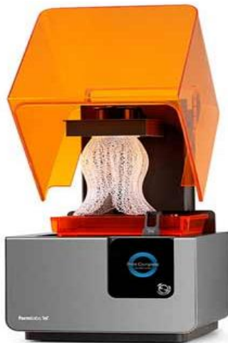
Obr. 8 3D tisk. Formlabs Form2 [14]
