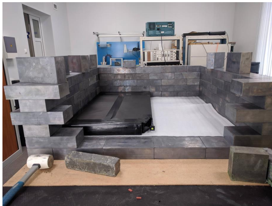
Figure 4-6 Gamma catcher scintillator
