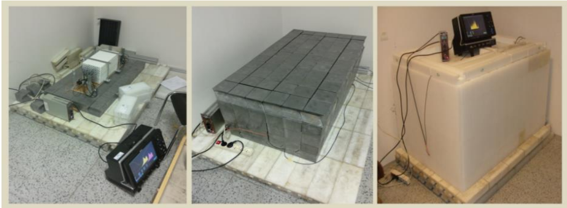
Figure 4-4 Construction of the scubino detector
