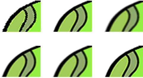
Figure 9: From left to right, top to bottom: deformation result is rendered by GL_NEAREST , GL_LINEAR , triangle, B-spline, bell, and Catmull-Rom texture filtering methods.
