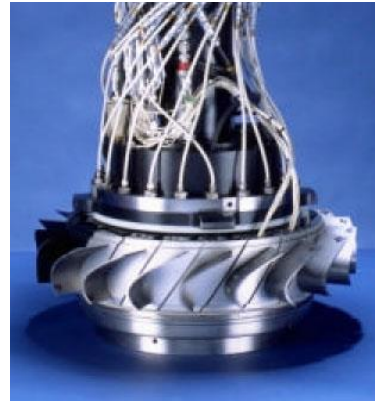
Figure 19 Annular cascade for traveling wave mode and influence coefficient testing
