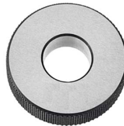
Fig. 2: The calibration ring measured by contact scanning at a speed of 8 mm/s with the step between points 0.1 mm (approx. 400 points). The diameter of the calibration ring was evaluated. The nominal size of the calibration ring is 39.9979mm.
