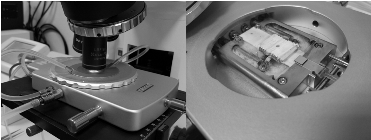
Fig. 1 The chamber during heating to higher temperatures (left), a view inside the chamber with a specimen on a ceramic glass (right) [4]
