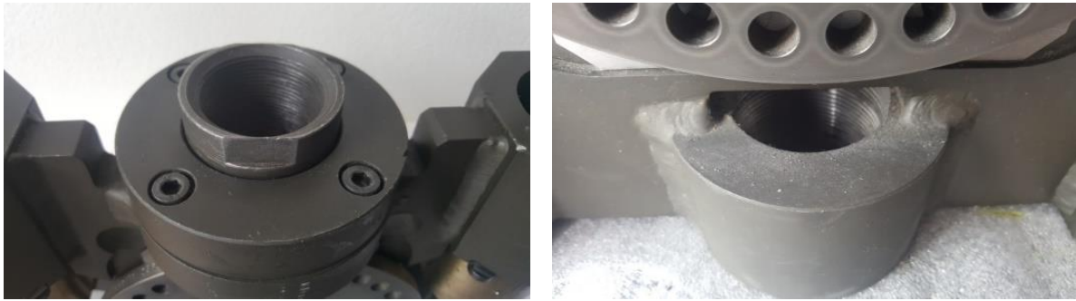
Fig 18- Connection nuts of the equipment
