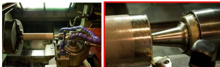
Stellite 6 - RINGN43-LX11-TUNGALOY Vc=250 m/min f=0.025 mm/rev ap=0.1 mm
