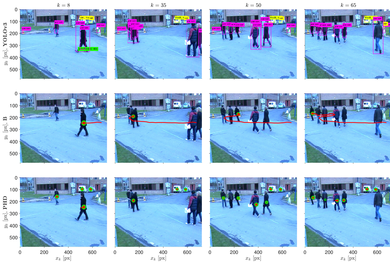
Fig. 6.12: Sample frames from View_006_T12-T34 video: YOLOv3, Bernoulli and PHD filters.
