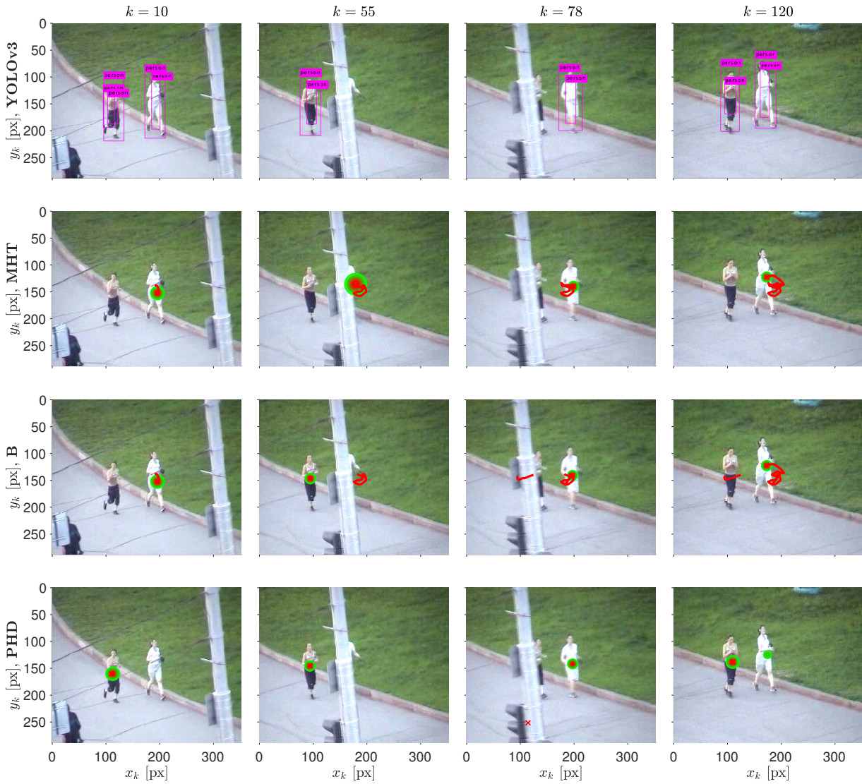
Fig. 6.10: Samples from Jogging video: YOLOv3, MHT, Bernoulli and PHD filters.
