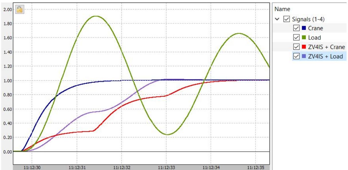
Figure 3.4: Comparison of simulation results with the same timeframe to show how effective input-shaping can be
