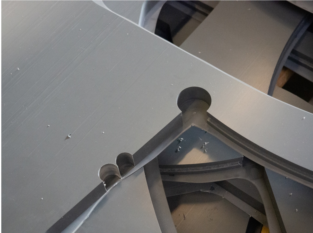
Figure 26: Manual cut out of the flat-shaped pieces
