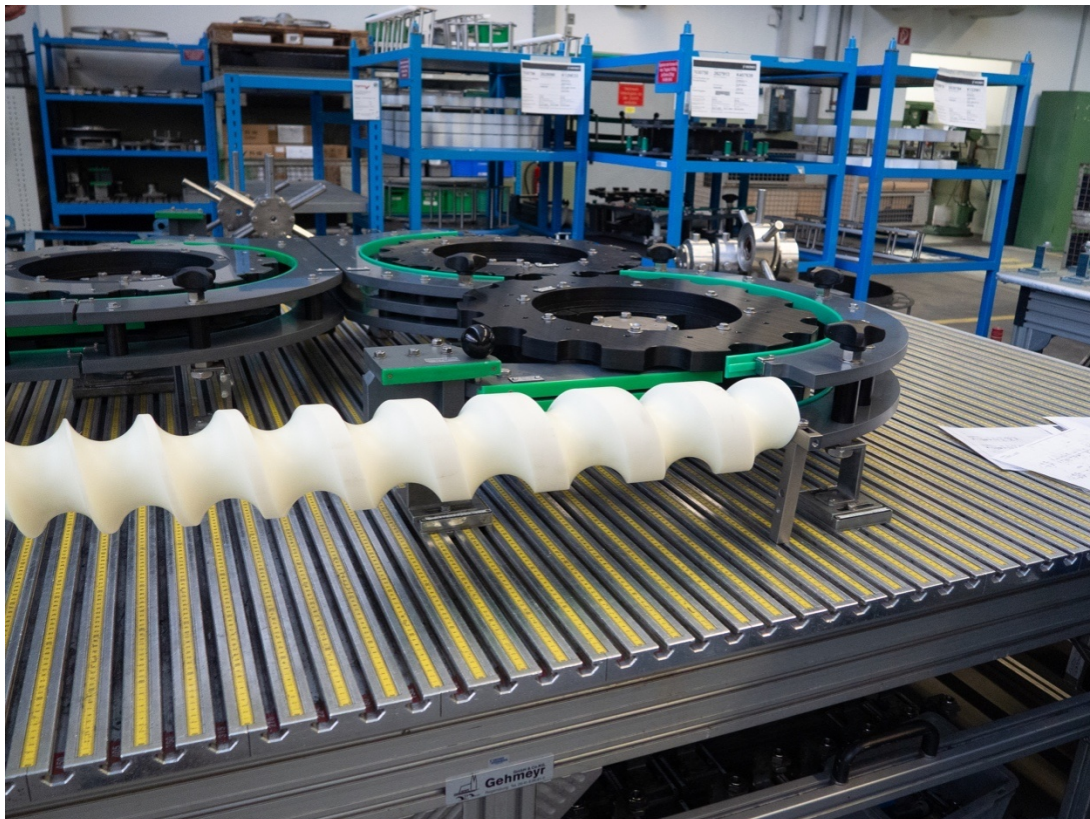
Figure 30: Pre-build container guiding system on the test table
