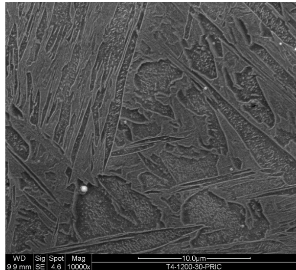
Obr. 5.11: T4 – 1200 – 30 – martenzit, dolní bainit
