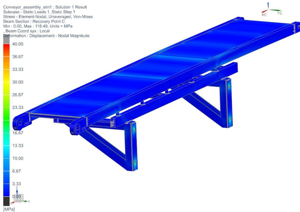
Figure 67 RESULTS: Stress - Element - Nodal (Von Mises)
