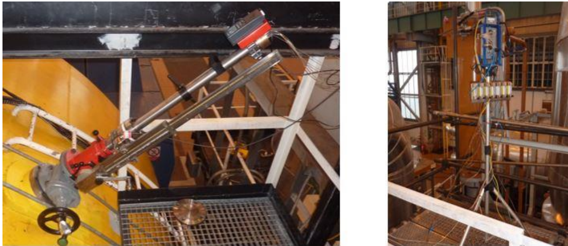
Figure 21. Overview of the probe stuck through the outer casing reaching the bottom of a blade [left]. Transducer and water droplet separators set at the top of a rack [right]. [15]
