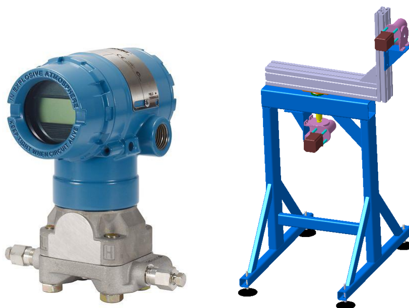
Figure 3. Pressure transmitter ROSEMOUNT [13] [left] and the probe stand [15] [right].
