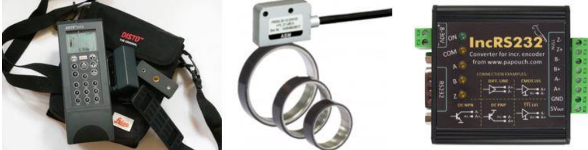
Figure 10. The rangefinder, the magnetic position encoder, the impulse counter. [15]
