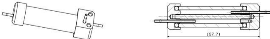
Figure 8. Design of customized water droplet separator. [15]
