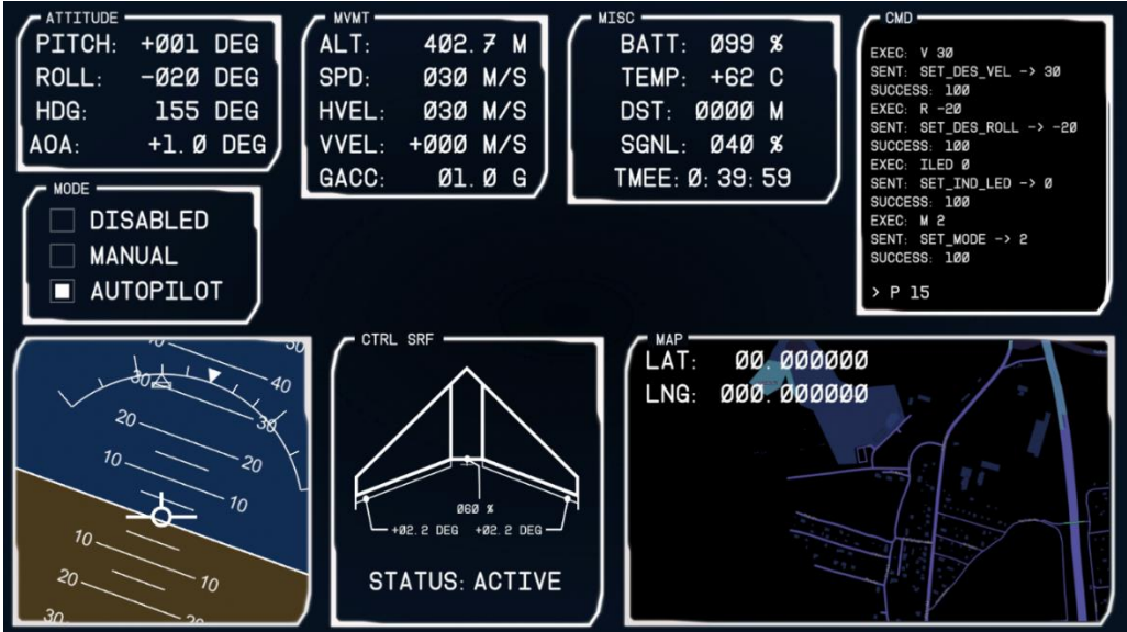
Figure 9: Ground control layout
