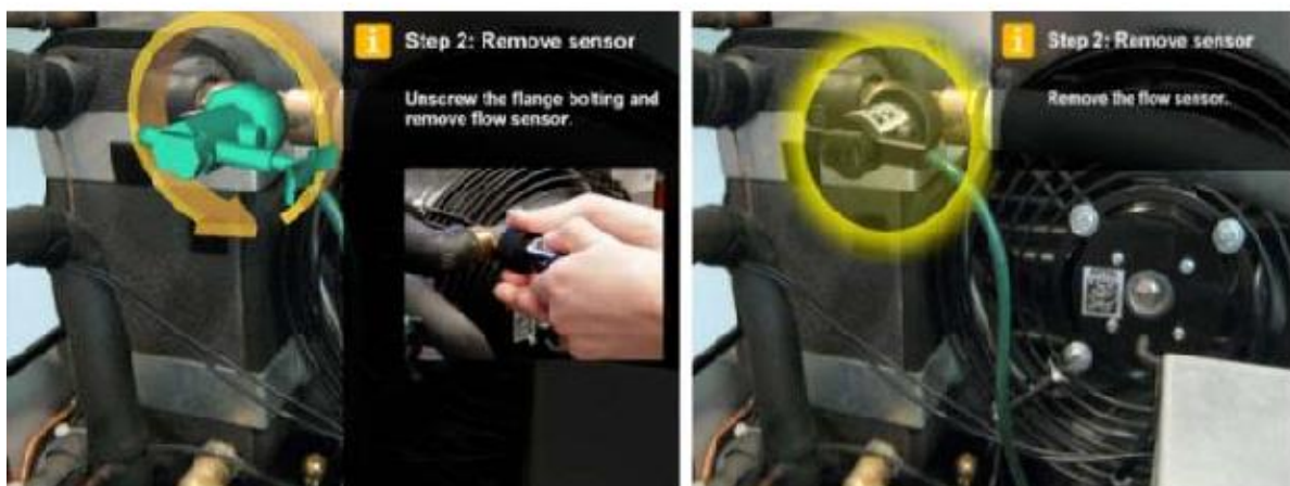
Figure 4 - Assembly and Maintenance Workflow with AR
