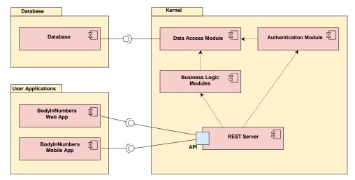
Figure 1. The component model of the BodyInNumbers system. It consists of three subsystems: kernel, database, and user applications. These subsystems consist of software components.
