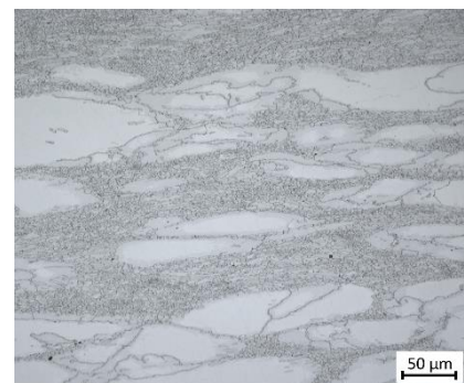
Figure 14. Microstructure produced by heating to semi-solid state and subsequent deformation - sequence 4 - reduction 3.
