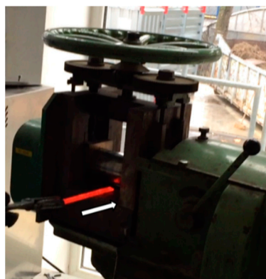
Figure 1. Rolling the heated container on the laboratory rolling mill.
