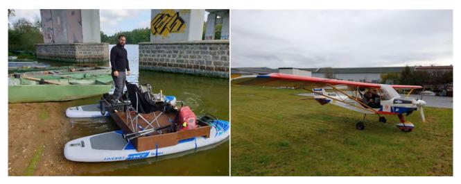
Figure 2 Plattform used for bathymetric survey and small aircraft used for photogrammetrical and LiDAR survey
