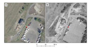
Figure 3 Example of Ground Control Point identification. A – contemporary orthophoto available as WMS. B – processed orthophoto from 2008.
