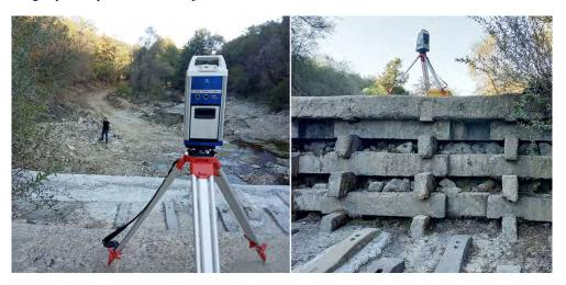
Figure 2. Stonex X300 laser scanner at operation in Damdere debris area
