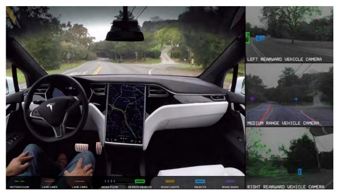
Figure 1. The interior of a driverless car and the road objects detected by the cameras (The Tesla Team 2016)
