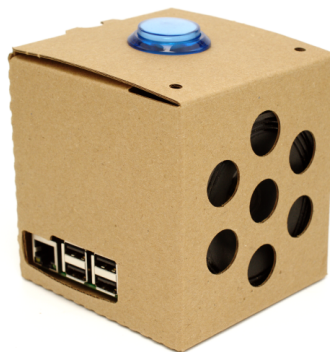
Figure 3.5: Photo of the assembled VoiceKit [10]
