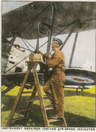
INSTRUMENT REPAIRER TESTING AIR-SPEED INDICATOR
