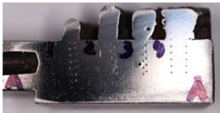
Fig. 4: Points at which hardness was measured.
