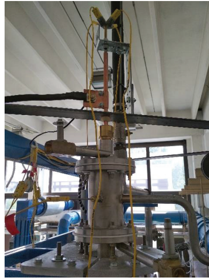
FIGURE 2. Output head with a mobile thermocouple.
