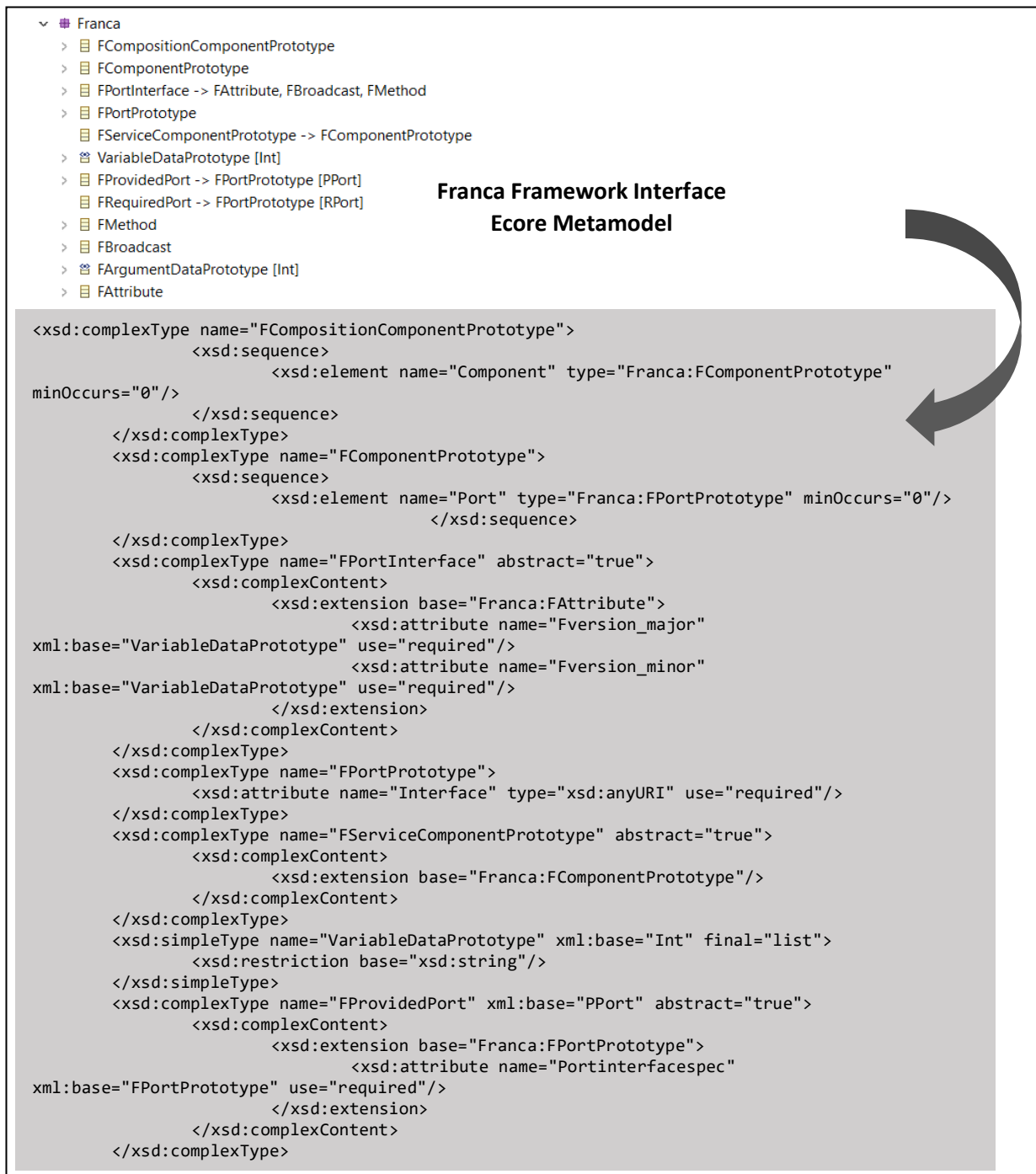
Fig. 66. An example on exporting ecore metamodel constructs to equivalent XML schema using emf tools.
