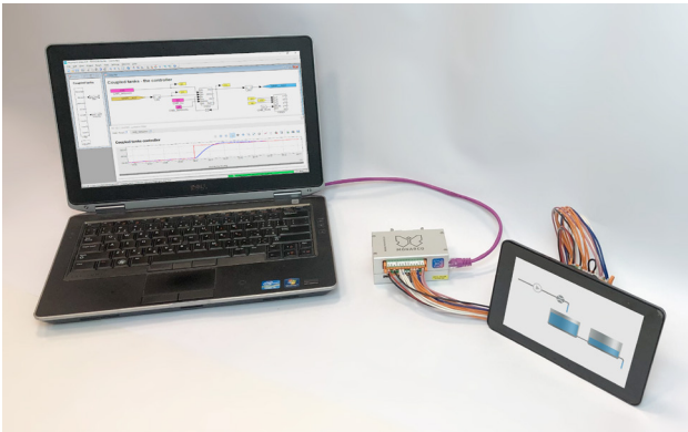
Fig. 4. Engineering station (left), controller (middle) and the controlled plant (right)
