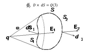
Pic.3 Different Gaussian surfaces with the same amount of electric field vector flux[3]
