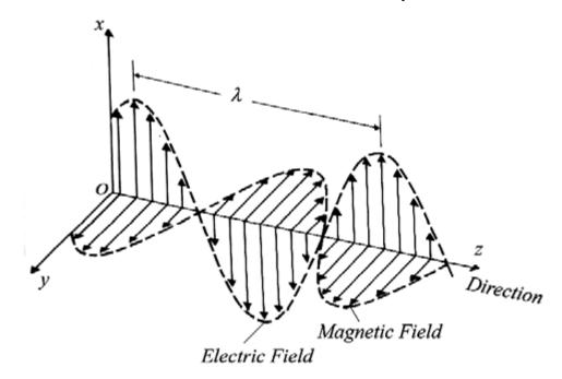
Pic.5 Propagation of electromagnetic wave in free space [5]
