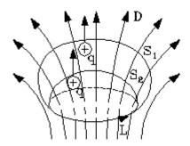
Pic.4 In an arbitrary magnetic field, two arbitrary surfaces are stretched on some contour[4]
