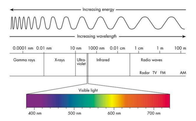
Pic.6 Electromagnetic spectrum[6]
