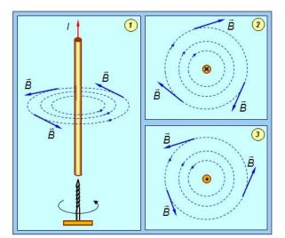
Pic.1 Magnetic field lines of an infinitely long rectilinear conductor with current[1]
